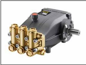
■ Rugged **High-Pressure Pump**, with three ceramic plungers, forged brass head and seven-year warranty, is connected to the engine by a belt-drive assembly that features cast-iron bushing **Pulleys** and two notched "V" cogged belts, which provide a cooler operation and longer life; also two-bolt adjustment makes it easy to adjust the belt tension.
